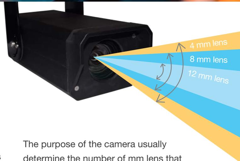
The purpose of the camera usually determine the number of mm lens that is needed. A camera with a 2.8 mm lens has a wider viewing angle, this camera will give a broader picture on the monitor but provides less detail. A camera with an 8 mm lens has a smaller viewing angle, but gives a lot of details. This applies to both horizontal and vertical angles.
